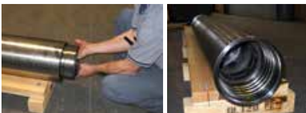
Bit bearing installed.
