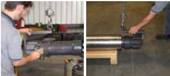
Lubrication and installation of the piston.
