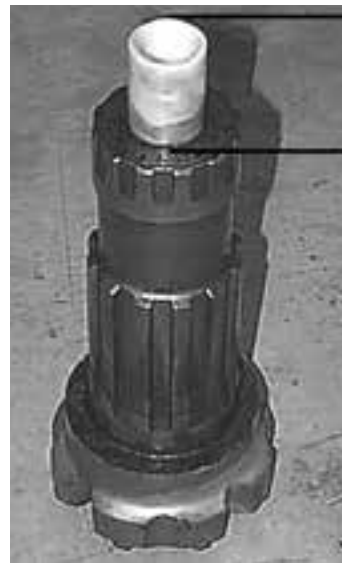
Correct exhaust tube extension
