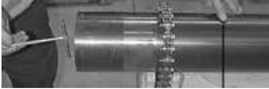
Measure at this point (1/2" past long undercut)
