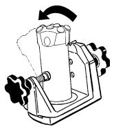
Before grinding, always check that there are no traces of explosive in the flushing holes of the drill bit. Clamp the drill bit securely in the holder. Use the right bit holder for the size and thread of the drill bit. To grind the gauge buttons, incline the holder to the correct angle so that the button is vertical during grinding.
