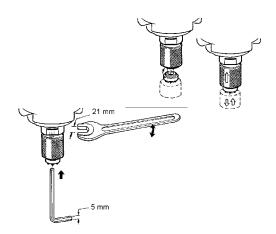
Before fitting the grinding cup, smear the shaft of the cup with a rust-inhibiting agent such as Shell Ensis Compound 356 or similar.
