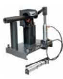
It is always most convenient to break the hammer threads on the rig. For circumstances, when the threads cannot be broken or tend to get stuck, there is a breakout bench available.
