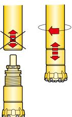
DTH hammers must be rotated to the **RIGHT** (clock wise) during drilling, since the driver chuck and top sub are threaded into the cylinder with **RIGHT-HAND THREADS**.
