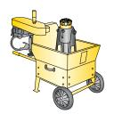
The Grind Matic Manual B-DTH is a mechanized air-powered grinding machine for button bits. It is mounted in a steel box-barrow, which can be wheeled easily around the worksite. The Grind Matic Manual B-DTH uses diamond-impregnated grinding wheels.
