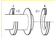
The buffer rings must be mounted with their concave (curved) surfaces towards the control tube flange. Incorrectly fitted buffer rings can cause serious damage to the hammer.
