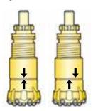
Since the driver chuck and hammer cylinder are "sand-blasted" continuously by large volumes of abrasive cuttings during drilling, they eventually become worn out. The areas adjacent to the cuttings grooves in the drill bit will be subjected to the most wear. To prevent uneven wear of the hammer cylinder, therefore, the driver chuck and bit should be marked as shown in figure, before the chuck is lifted off the bit.
