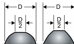
Button bits should be regrind when the penetration rate drops, or if any of the cemented carbide buttons are damaged (fractured buttons should be ground flat). It is both practical and economical to redress the buttons when
