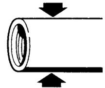
The outside diameter of the driver chuck must not be less than that of the hammer cylinder.
