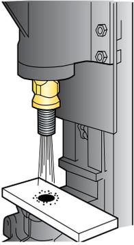
Lubricating oil is vital for the satisfactory operation of DTH hammers. Apart from regular checking of the oil level in the lubricating-oil tank, always make sure that there is oil in the compressed air. This can be checked whenever the rotation unit is free, i.e. disconnected from the drill string.
