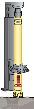
Run the hammer into the rock or a thick plank.
