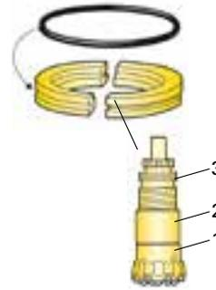
Make sure the stop ring is located correctly, and that it faces the right direction. Incorrect fitting will result in severe damage to the hammer.
