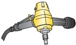
The Grind Matic HG is a portable, hand-held, air-powered grinding machine for button bits, ideal for use at the worksite. It is used with diamond-impregnated grinding cups, which can be used with or without water flushing.
