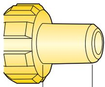
After fitting the foot valve into the bit shank, its protrusion from the end of the shank must be checked. Too much or too little protrusion will seriously affect the performance of the hammer.
