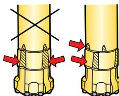
When fitting the driver chuck back on to the drill bit after grinding or replacing a drill bit, its radial location on the bit shank should be advanced by one spline section. This will give a more even distribution of wear on the driver chuck and hammer cylinder.
