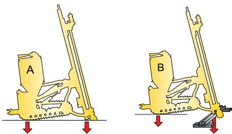
Before drilling with the DTH hammer, the rig must be set-up correctly in order to give stability and safety. If this is not done, the effects of feed force and rotation torque can cause
