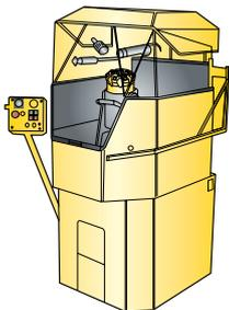
For "permanent" grinding stations, a mechanized stationary grinding machine is available, the Grind Matic BQ3-DTH. It is equipped with automatic feeding devices and grinds both the cemented-carbide buttons and the bit-body steel in one operation. The machine uses diamond-impregnated grinding wheels.
