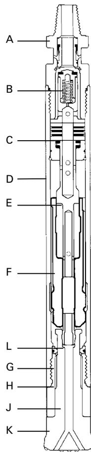
The splined union between the driver chuck **K** and bit shank **J** transmits rotation to the drill bit. The front end of the driver chuck transmits feed force to the drill bit. The split stop ring **H** limits axial movement of the drill bit. The check valve **B** prevents water from entering the hammer through the driver chuck when the compressed air supply is shut off.
