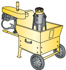
The Grind Matic Manual B-DTH is a mechanized air-powered grinding machine for button bits. It is mounted in a steel box-barrow, which can be wheeled easily around the worksite. The Grind Matic Manual B-DTH uses diamond-impregnated grinding wheels.
