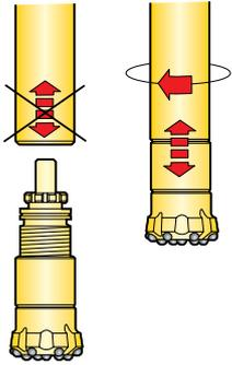
DTH hammers must be rotated to the RIGHT (clock wise) during drilling, since the driver chuck and top sub are threaded into the cylinder with RIGHT-HAND THREADS.
