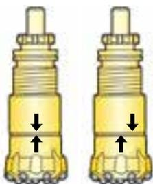
Since the driver chuck and hammer cylinder are "sand-blasted" continuously by large volumes of abrasive cuttings during drilling, they eventually become worn out. The areas adjacent to the cuttings grooves in the drill bit will be subjected to the most wear. To prevent uneven wear of the hammer cylinder, therefore, the driver chuck and bit should be marked as shown in figure, before the chuck is lifted off the bit.
