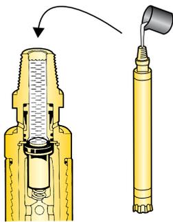
The sealing efficiency of the check valve can be checked by pouring a small quantity of lubricant through the top sub of the hammer, with the hammer held vertical. If the lubricant passes through the check valve, then the valve spring and/or valve seal is worn or damaged and should be replaced immediately.
