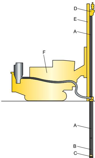
Secoroc COP down-the-hole hammers are designed for use on DTH or ITH drill rigs. They can also be used on rotary and auger type drill rigs, provided that such rigs meet the specifications for DTH applications. The main demands on the drill rig are as follows:
