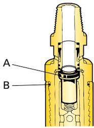
All Secoroc COP down-the-hole hammers contain a check valve that is designed to trap a quantity of air inside the hammer when the air supply is switched off. In most conditions, this prevents the ingress of water and dirt into the hammer during jointing operations. The check valve A and O-ring B must be fault-free when drilling in water-bearing formations. When drilling deep holes in rock with a high water inflow, however, it is possible that
