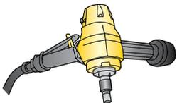
The Grind Matic HG is a portable, hand-held, air-powered grinding machine for button bits, ideal for use at the worksite. It is used with diamond-impregnated grinding cups, which can be used with or without water flushing.
