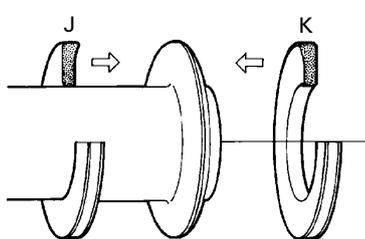
The buffer rings must be mounted with their concave (curved) surfaces towards the control tube flange. Incorrectly fitted buffer rings can cause serious damage to the hammer.
