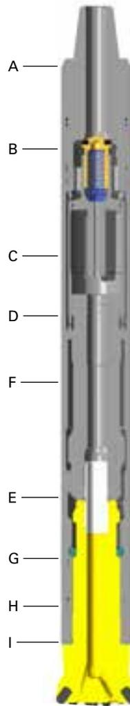
The COP W4 hammer has a long casing **D**, which houses a check valve **B**, impact piston **F**, exhaust tube **E**, retaining ring **G** and drill-bit shank **H**. The back end of the cylinder is closed by a threaded backhead **A**. The backhead has a male thread for connection to the drill pipes, and is provided with wrench flats.
