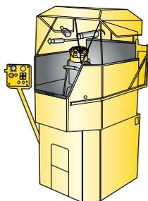
For permanent grinding stations, a mechanized stationary grinding machine is available, the BQ3-DTH. It is equipped with automatic feeding devices and grinds both the cemented-carbide buttons and the bit-body steel in one operation. The machine uses diamond-impregnated grinding wheels.
