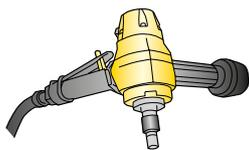
The grinding machine HG is a portable, handheld, air-powered grinding machine for button bits, ideal for use at the worksite. It is used with diamond-impregnated grinding cups, which can be used with or without water flushing.
