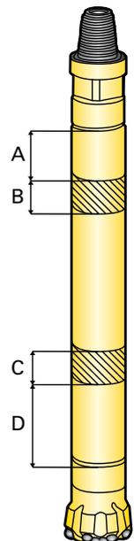
If special tools like chain wrenches or other types of wrench are used to break the hammer joints, then the tool must be attached around the hammer cylinder as shown in the figure. Do not attach at other points!
