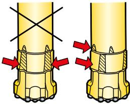
When fitting the driver chuck back on to the drill bit after grinding or replacing a drill bit, its radial location on the bit shank should be advanced by one spline section. This will give a more even distribution of wear on the driver chuck and hammer cylinder.
