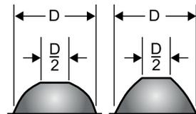
Button bits should be reground when the penetration rate drops, or if any of the cemented carbide buttons are damaged (fractured buttons should be ground flat). It is both practical and economical to redress the buttons when the wear flat reaches about 1/2 of the diameter of the button.
