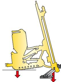
When drilling in soil or other non-consolidated formations, the weight of the rig must not be loaded on to the feed near the mouth of the hole, since this could easily cause the hole to cave-in. Instead, the load should be distributed some distance to either side of the hole. Suitable support can be obtained by placing a sturdy U-beam under the base of the feed beam, and supporting the beam on planks at both ends. A two inch (50 mm) plank should then be placed inside the U-beam
