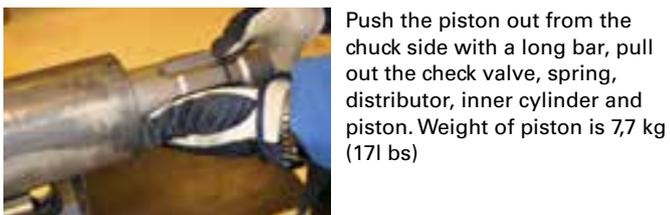
Push the piston out from the chuck side with a long bar, pull out the check valve, spring, distributor, inner cylinder and piston. Weight of piston is 7,7 kg (17l bs)
