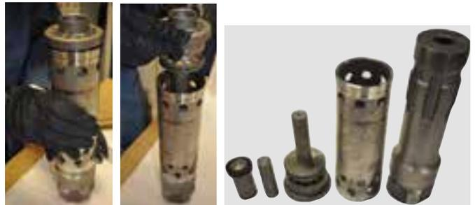
Remove the inner cylinder from the distributor. A preferred method is to take the inner cylinder and distributor and fit it over the small diameter end of the piston. By raising the assembly up and impacting it down onto the piston, the inner cylinder can be freed. Be careful not to get fingers caught in the cross holes in the inner cylinder while driving it up and down.
