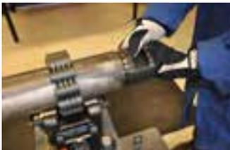
Lubricate the assembly with hammer oil and slide it into the backhead end. Smear the backhead thread with thread grease, tight backhead by hand.
