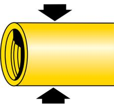
Wear to the driver chuck and hammer cylinder should be checked regularly, e.g. every time the bit is reground or changed. Measure the diameter of the hammer cylinder using a sliding calliper. Measure along the full length of the cylinder, with the exception of the outermost 100 mm at each end. At any point between these points, the diameter of the hammer cylinder must not be less than the minimum permissible diameter given for the respective DTH hammer sizes in the table below.
