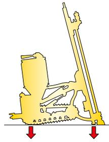
When setting up a drill wagon or crawler drill rig, a stable three-point set-up must be obtained, with the weight of the rig distributed between the base of the feed beam and the two rear corners of the rig. It is of the utmost importance that the rear loading points are as far to the rear of the rig as possible, with most of the rig weight being loaded on to the base of the feed.
