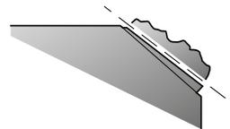
A drill bit can remain in service as long as the gauge buttons maintain the diameter of the bit. Fractured buttons must always be ground flat to prevent chips of cemented carbide from damaging the other buttons.
