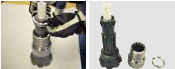
Remove bit retaining ring and chuck from drill bit.
