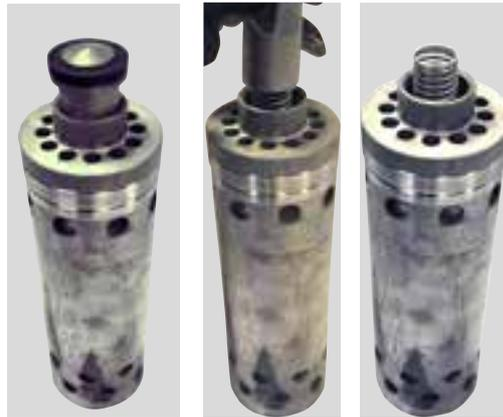
Remove check valve and spring from distributor.
