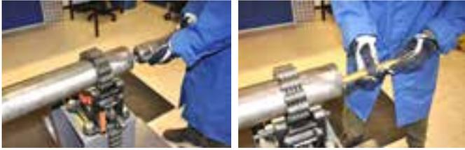
Inspect the piston for wear or cracks, replace if cracks are found. Lubricate the piston and casing inside with hammer oil and install the piston from the backhead side of the casing with a brass bar.
