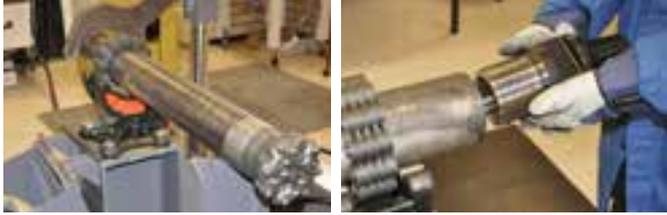
Remove backhead. Backhead thread connection need to be loosened up with a breakout-bench. Lift out the backhead, weight of the backhead is around 7,4 kg (16,3 lbs).
