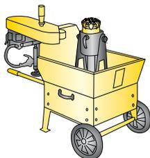
The grinding machine Manual B-DTH is a mechanized air-powered grinding machine for button bits. It is mounted in a steel box-barrow, which can be wheeled easily around the worksite. The Manual B-DTH uses diamond-impregnated grinding wheels.
