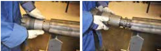
Remove drive chuck, drill bit and bit retaining ring. Chuck thread connection need to be loosened up either with breakout table on drill rig before hammer is removed or with a breakout bench.
