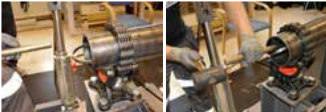
2) Place the lock ring in place by using a steel bar and hammer.
