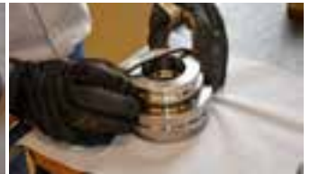
4) Lubricate the splines on the drill bit with thread grease, Install the driver chuck and bit retaining ring on to the drill bit with the thicker side of retaining ring facing upwards. Install the complete unit to the hammer, smear the chuck thread with thread grease and tight by hand.
