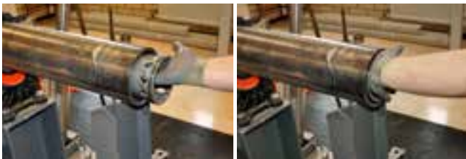
3) Inspect the bit bushing for wear or cracks. Lubricate the bit bushing with oil and place it in to the chuck side of the hammer. Knock the bushing in with a brass punch. Observe, the o-ring must be down to the chuck side of the hammer.
