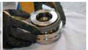
5) Clean the disc springs using a piece of cloth and check for cracks and damage. Smear the discs with grease and assemble them in the right sequence.
