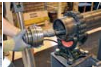
6) Smear and assemble the cover and control tube. Smear the cover unit and the control tube with COP oil. Push the control tube and cover from backhead side. Using a rod makes it easier to fit the control tube into the piston.
