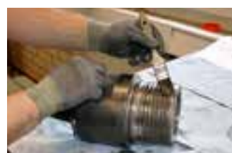
7) Lubricate the backhead thread with tread grease, tight back-head assembly by hand.
