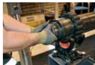
6) Smear and assemble the cover and control tube. Smear the cover unit and the control tube with COP oil. Push the control tube and cover from backhead side. Using a rod makes it easier to fit the control tube into the piston.
