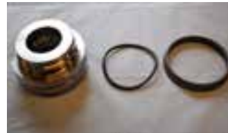
4) Lubricate the splines on the drill bit with thread grease, Install the driver chuck and bit retaining ring on to the drill bit with the thicker side of retaining ring facing upwards. Install the complete unit to the hammer, smear the chuck thread with thread grease and tight by hand.
