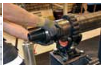
7) Lubricate the backhead thread with tread grease, tight back-head assembly by hand.
