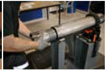
4) Lubricate the splines on the drill bit with thread grease, Install the driver chuck and bit retaining ring on to the drill bit with the thicker side of retaining ring facing upwards. Install the complete unit to the hammer, smear the chuck thread with thread grease and tight by hand.
