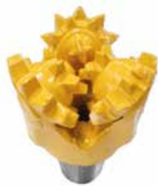
TCI bits have inserts placed into the steel cones (similar to DTH Bits), the size and shape of the inserts, dictating the kind of formations to be drilled. Often used for drilling harder igneous formations, especially with hemi-spherical inserts.
