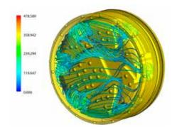
Flow simulation in the Elemex face design.
