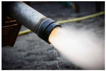
The extended ring bit wall of the Elemex system redirects the air within the drilling area. This decreases the air pressure just enough to get an efficient flushing. The intensity of the air that reaches the surrounding soil is significantly lower.
