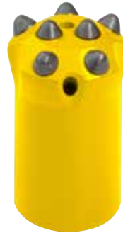
Model -17 All-round drill bit for soft to medium-hard rock. Front and side flushing. Diameters up to 34 mm.
