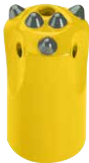
Model -12 This bit is used in medium to hard rock formations. One front flushing hole and two side flushing holes.
