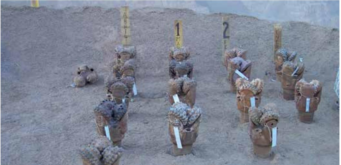
At many mines, the decision regarding when to change the bit is left up to the driller, with very little guidance given. This results in most bits being changed only after they have been completely worn out, and when they have been operating at low efficiency for a length of time. You can save a great deal of money by establishing a program of close examination and grading of your used bits, and by applying some simple rules based on this information.
