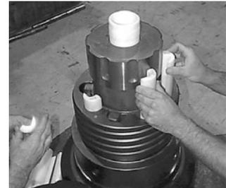
11. Install the bit retaining rings and bit retaining ring o-ring on to the bit and chuck.
