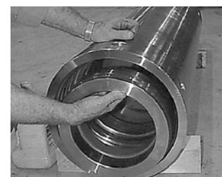
11. With the casing standing vertically (the backhead end up and the chuck end down), the **piston can be used to drive the bearing retaining ring from the casing**. A brass bar may be useful for impacting and driving the piston. The plastic non-lube bearing retaining ring can be removed by hand. This may make field replacement of seals easier.
