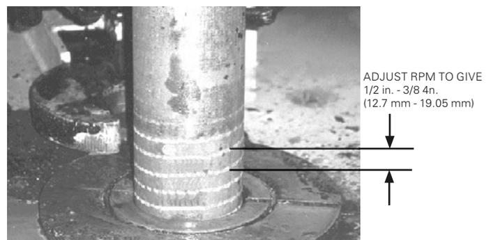
Another method for setting rotation speed involves witnessing the wear flat developed on the carbide. The wear flat on the should be directly on the top of the inserts. A flat which is on the leading edge of carbide (side facing the direction of rotation) indicates rotation speed is too slow. Conversely, rotating too fast will cause rapid wear of the bit and the wear flat will be on the trailing edge of the carbide.
