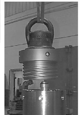
7. Install the piston through the chuck end of the casing.
