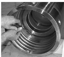
10. Coat the bit splines liberally with copper or zinc based thread compound and install the chuck on the bit.
