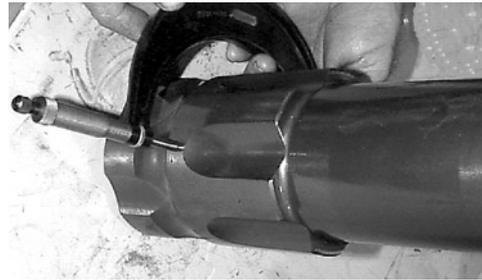
**12a Non-lube piston, seals and bearing inspection**
