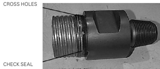
8. Inspect the check seal for erosion or damage, replace if necessary.
