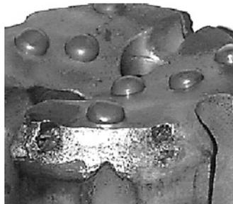
View showing wear flat on leading edge - indicates rotation too slow. note that carbide failure was caused by the leading edge wear flat.
