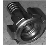
9. Inspect the **air distributor stem** (valve cap side) for grooving or severe corrosion where the valve seal contacts. Clean this area as required with emery paper to remove rust, scale or nicks and burrs. A distributor with a deep groove should be replaced.
