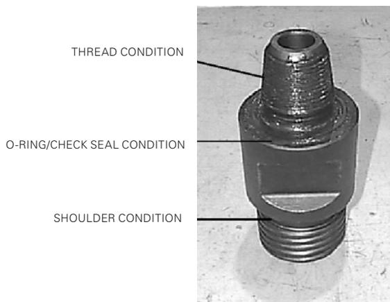
4. The **backhead o-ring or check seal** should be replaced if damaged in any way.
