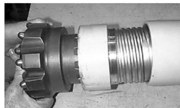
■ On the QL200 use a lifting bail on the backhead thread to lift the assembly and thread it onto the chuck.
