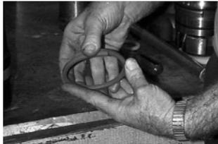
Install bearings and seals by spreading over groove and allowing them to snap back into undercuts.
