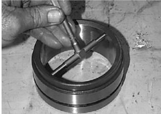
12. Inspect the **piston** for wear using micrometers in the four locations noted below. The piston usually wears more than its mating parts so it's likely that it will affect clearance the most. Record the dimensions for comparison to mating parts (cylinder, distributor and casing) to determine which part offers the most economical replacement cost. See special notes for non-lube seal and bearing inspection on page 3-23.
