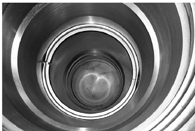
3. On the QL200 special handling is needed to install the cylinder assembly:
