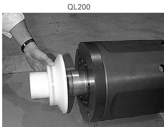
10. Moving back to the chuck end, **pull the bit bearing** from the hammer casing. Depending on the degree of rust or dryness of this area, a bearing puller may be needed to remove the bearing. When using a puller, be careful not to catch the bearing retaining ring. Sometimes lifting and dropping the casing on a block of hardwood can jar the bearing loose.
