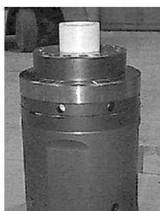
2. If the casing needs to be reversed, slide the cylinder, distributor and valve cap assembly into what was the chuck end. Otherwise slide the assembly into the backhead end. Note that even though the casing may not require reversal due to OD wear, it may be worthwhile to reverse the casing to renew the end of the bore the piston slides in. On the QL50/QL55QM, QL60/QL65QM and QL80 the cylinder stop ring in the casing does not need to be moved.
