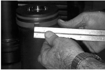
It is useful to pre-stress the seals slightly so they don't get caught in casing grooves when installing piston.
