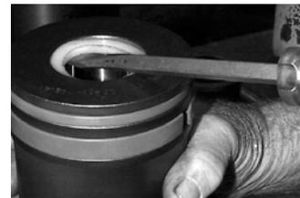
Install new tail seal by working it into the groove as much as possible.
