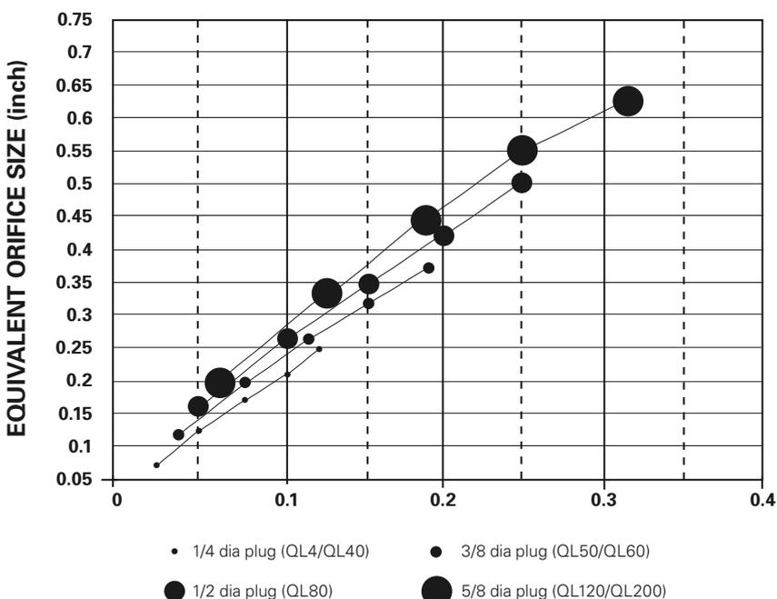
1. Diameter is based on flow entering from both sides of the flat (ie. two flats make up hole equivalent).
