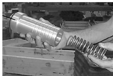
6a. **Remove the make up spacer, or on the QL200 bellville springs and make up spacer.**
