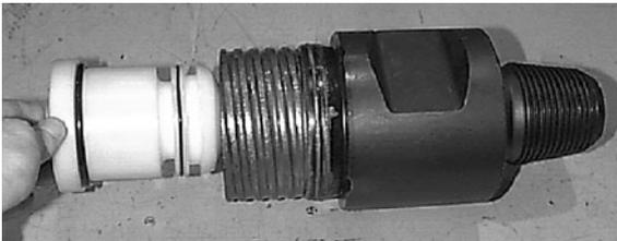
3. There is no need to remove **the inducer** unless damage is visible. **(Only inducers with snap rings can be removed).**
