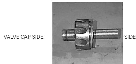
10. Inspect the **valve** for seal interference and damage. The valve seals should have interference with the valve cap bore and distributor guide. The valve sealing surfaces should be free of nicks and burrs.
