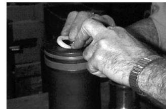
Snap tail seal into bore by lightly tapping into groove.
