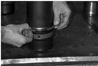
13. Carefully remove any sharp edges, burrs or nicks which have developed on the piston using a hand grinder. **Do not overheat the piston...it will crack if overheated!** If the piston face is heavily cavitated or pitted either use a ceramic facing tool to dress the face of the piston or use a well cooled grinder. In either case, a maximum of .060 in. (1.52 mm) can be removed from the piston face.
