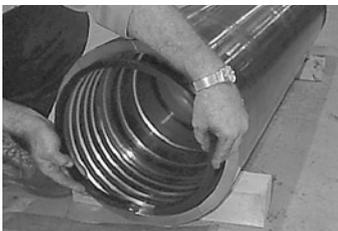
9. Insure the o-ring on the bearing is in good shape as it holds the bearing in place when the chuck is removed. Slide the bearing into the casing until it seats against the bearing stop ring. The bearing may need to be tapped from side to side to prevent it from getting stuck in the bore.
