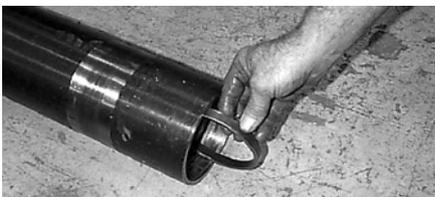
■ On the QL120/QL200 install the polyurethane bearing stop ring in the groove by hand.
