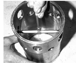
16. Inspect the **air distributor** for excessive wear on the valve seat, replace if wear is deeper than .005 in. (.127 mm). Measure and record the guide diameter for later reference.
