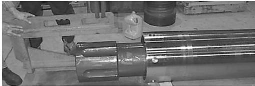
8. Install the bearing stop ring into the casing by starting it sideways and when it is near the undercut turn into the proper orientation until it snaps into the groove. **Be sure to wear safety glasses as oil and grease in the groove may be expelled when the ring snaps.**
