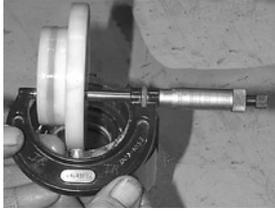
11. Inspect the **bearing bore** just above the internal flutes for wear using a telescopic bore gage and a micrometer. Replace the bearing if the net clearance with a new bit has worn beyond the discard point. Replace the bearing o-ring if it has been damaged or torn.
