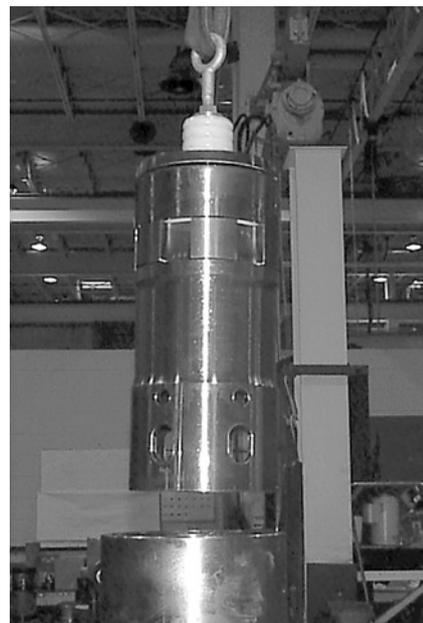
8. **Disassemble the cylinder assembly** by prying the valve cap from this air distributor. An old set of belleville springs are sometimes useful for prying the valve cap from the distributor. Be careful not to damage the valve when prying the cap off.
