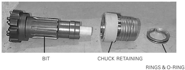
4. Remove the chuck from the bit.
