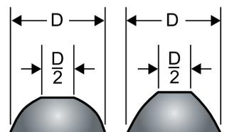
Button bits should be regrind when the penetration rate drops, or if any of the cemented-carbide buttons are damaged (fractured buttons should be ground flat). It is both practical and economical to redress the buttons when the
