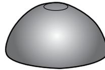
Do not grind too much on the top of the buttons. Let a few millimetres of the wear flat remain on top of the button.
