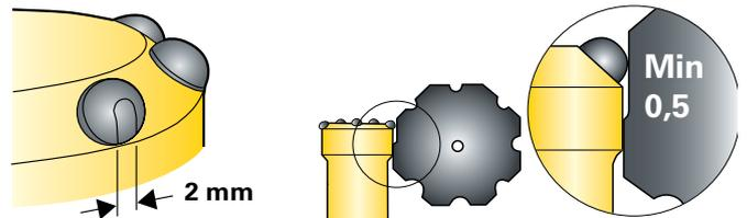
Gauge button anti-taper has to be removed by grinding, although excessive reduction of the bit diameter should be avoided. Leave about 2 mm of the wear flat. If necessary, remove some of the bit-body steel below the gauge buttons, so that a clearance (taper) of 0,5 mm is maintained. If the flushing holes start to deform, open them up with the aid of a rotary burr or steel file.
