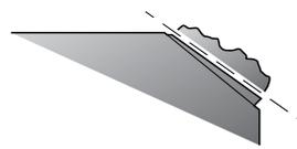
A drill bit can remain in service as long as the gauge buttons maintain the diameter of the bit. Fractured buttons must always be ground flat to prevent chips of cemented carbide from damaging the other buttons.
