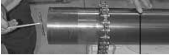
Measure at this point (1/2" past long undercut)
