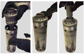
Place the distributor over the inner cylinder and drive the distributor until all faces mate. Install the check valve and the spring on it.
