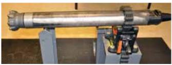
It is most important that the lock halves are fitted properly. The halves are broken to keep exactly the right size and shape. Make sure that the individual marking always stays in the same direction to keep the two ends perfectly matched.
