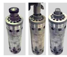
Remove check valve and spring from distributor.
