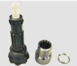
Remove bit retaining ring and chuck from drill bit.
