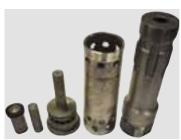
Remove the inner cylinder from the distributor. A preferred method is to take the inner cylinder and distributor and fit it over the small diameter end of the piston. By raising the assembly up and impacting it down onto the piston, the inner cylinder can be freed. Be careful not to get fingers caught in the cross holes in the inner cylinder while driving it up and down.
