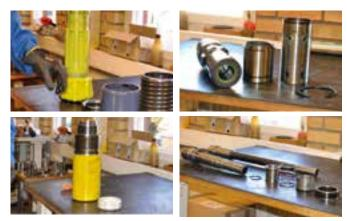
11). Check and inspect all components of the hammer. Replace O-rings, worn out and/or damaged items.
