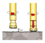
With holes of relatively shallow depth, the setting of feed and rotation is usually a simple matter in DTH drilling, since the hammers are comparatively insensitive to small variations in the "normal" flow and pressure settings. The settings can be regarded as correct when the drill string turns evenly without jerks or jamming, and a steady penetration rate is obtained.
