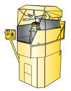
For "permanent" grinding stations, a mechanized stationary grinding machine is available, the Grind Matic BQ3-DTH. It is equipped with automatic feeding devices and grinds both the cemented-carbide buttons and the bit-body steel in one operation. The machine uses diamond-impregnated grinding wheels.
