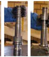
10. Remove the check valv assembly from the adapter tube.
