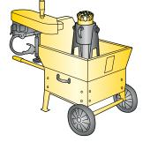
The Grind Matic Manual B-DTH is a mechanized air-powered grinding machine for button bits. It is mounted in a steel boxbarrow, which can be wheeled easily around the worksite. The Grind Matic Manual B-DTH uses diamond-impregnated grinding wheels.
