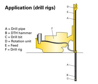
Secoroc RC hammers are designed for use on RC drill rigs. They can also be used on DTH, ITH, rotary and auger type drill rigs, provided that such rigs meet the specifications for RC applications. The main demands on the drill rig are as follows:
