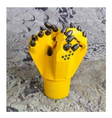
For drilling in soft rock, nothing beats the Altas Copco Secoroc Klaw bit. The Klaw bit is built from a solid piece of high grade steel, and uses tungsten carbide picks as its cutting structure. It is easy to replace these picks in the field in just a few minutes, essentially renewing the bit back to the new drilling condition.
