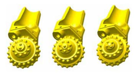
Bit kits are pilot bits that are used for building cutting tools, like hole openers, core barrels among others. The Atlas Copco bit kits are specially manufactured to have high quality bearing and cutting structures, without adding any unnecessary processes that might damage the vital features of the cutters.
