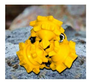
Atlas Copco has a large selection of milled tooth pilot bits for soft and unconsolidated ground formations. The pilot bits have an optimized shirttail protection, hard metal on the bevel, and inner rows of the cones to withstand the harsh drilling conditions that are typically encountered in the HDD application.
