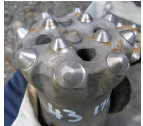
Norrtälje, Sweden. Powerbit T45, 76 mm retractor, with HD Trubbnos buttons. The Trubbnos profile is re-created after grinding, keeping a wear flat area of 10-20%.
