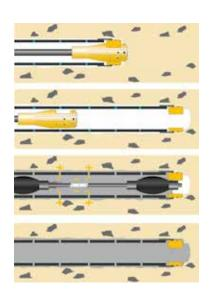
Cement grout is commonly used for filling the gap between the pipes and ground. A grout cap at the pipe mouth is used and backfill grouting applied. However, sometimes customers use pipes with one way injection valves for injecting grout with higher pressure providing improved grouting quality and further consolidated ground. In these cases, double packers might be utilized.
