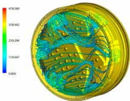
Flow simulation in the Elemex face design.
