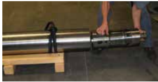
Installing the assembly in the hammer.
