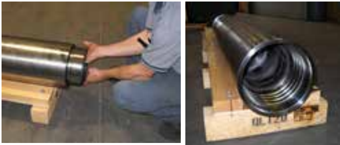
Bit bearing installed.
