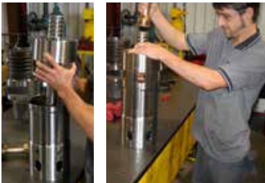
Installing the distributor in cylinder.
