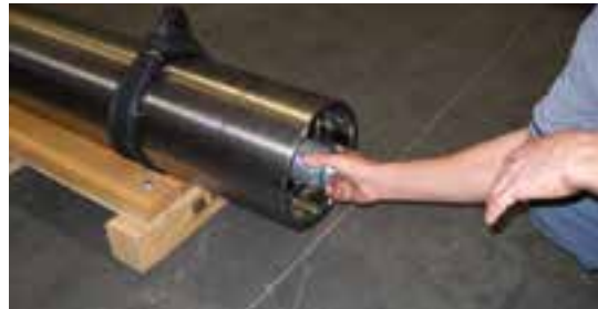
Installing check valve.
