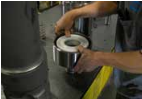
Installing the valve in the valve cap.
