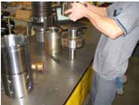
Installing the valve cap.
